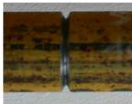
Fig. 6. The rod with the circumferential groove.
