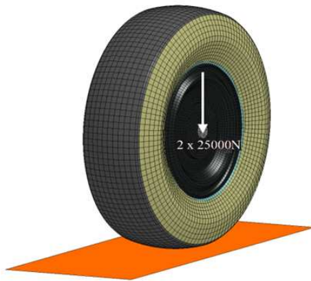
Fig. 12. Numerical model of the tire with applied force
