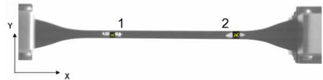
Fig. 5. An example of measurement points placing on a coupon with adopted coordinate system
