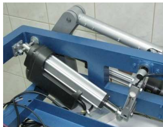
Fig. 8. Lifting drive with measuring beam
