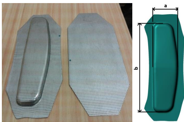
Fig. 1. Final shape and dimensions of the part and the blank
