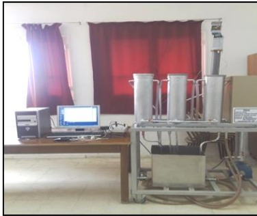
Fig. 4. Three tanks hydraulic system
