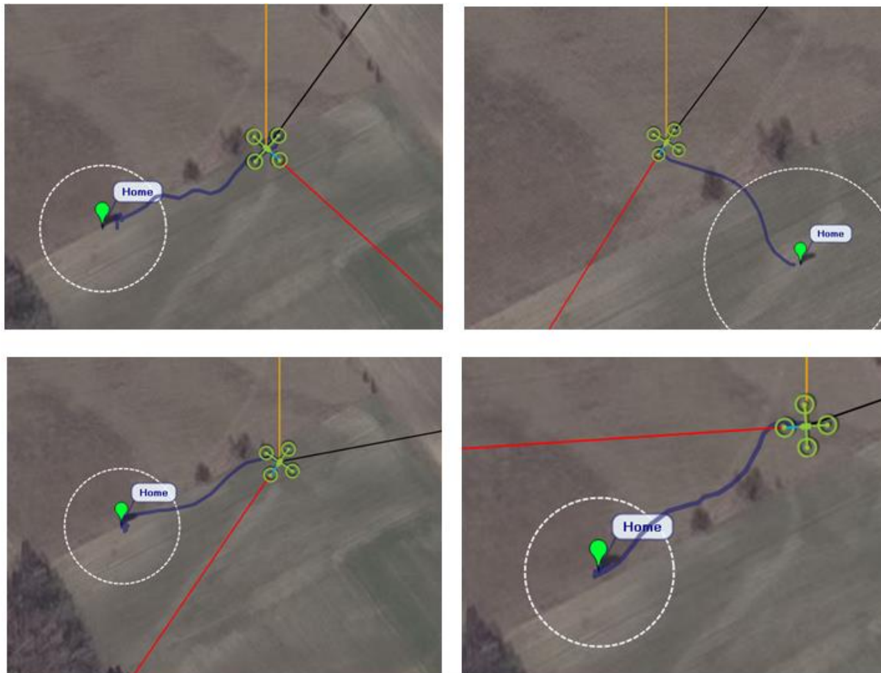
Fig. 10. Quadrotor flight paths during in-flight tests (based on the satellite maps of the investigated area)
