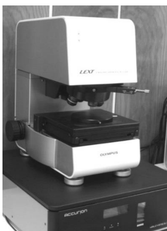
Fig. 5. Confocal microscope Olympus OLS 4000 Lext
