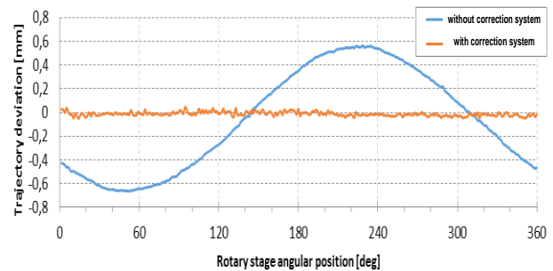
Fig. 8. Comparison of the head diversion from the position of the joint with active and inactive adjustment system (processing parameters: laser power 2kW, table rotation speed 45°/s)
