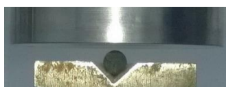
Fig. 8. Sample \varnothing 10 \times 42 on testing stand
