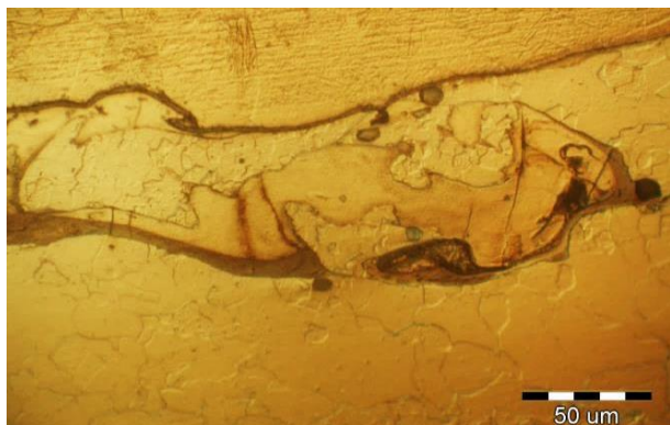
Fig. 12. Photo of joint area of one of tested bimetallic specimen before fatigue test
