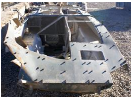
Fig. 3. AMV Rosomak after IED explosion (Slawinski's own resources, Afghanistan, 2012)
