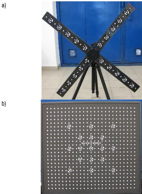
Fig. 3. The 5M PONTOS calibration devices: (a) cross; (b) plate
