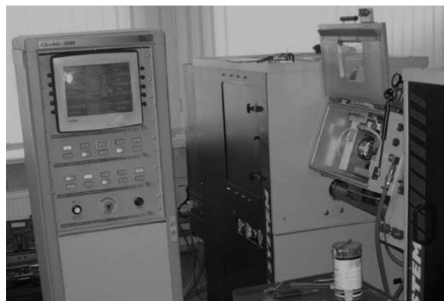
Fig. 5. Physical simulator Gleeble 3800, used in experimental research
