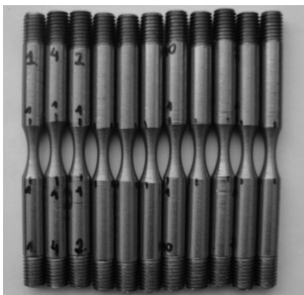
Fig. 6. A set of samples made of C45 steel used for experimental research
