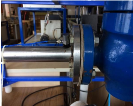
Fig. 5. Mounting of Accelerometer
