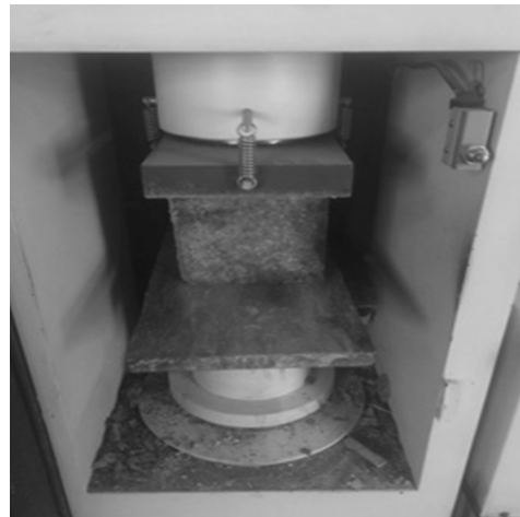
Fig. 9. Compressive strength testing in progress
