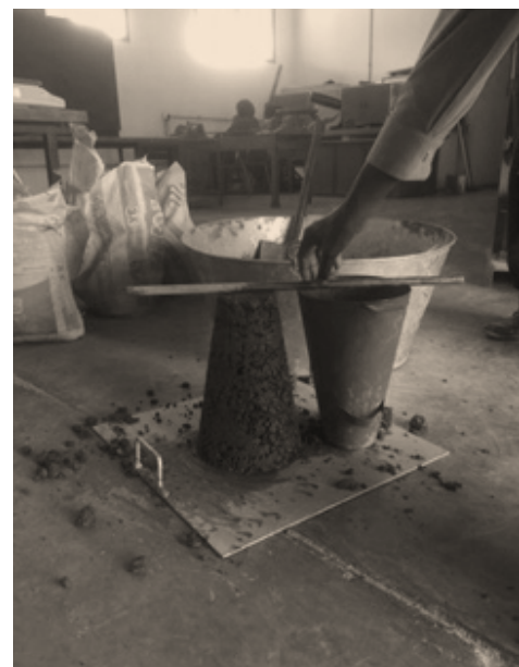
Fig. 6. Slump test in progress
