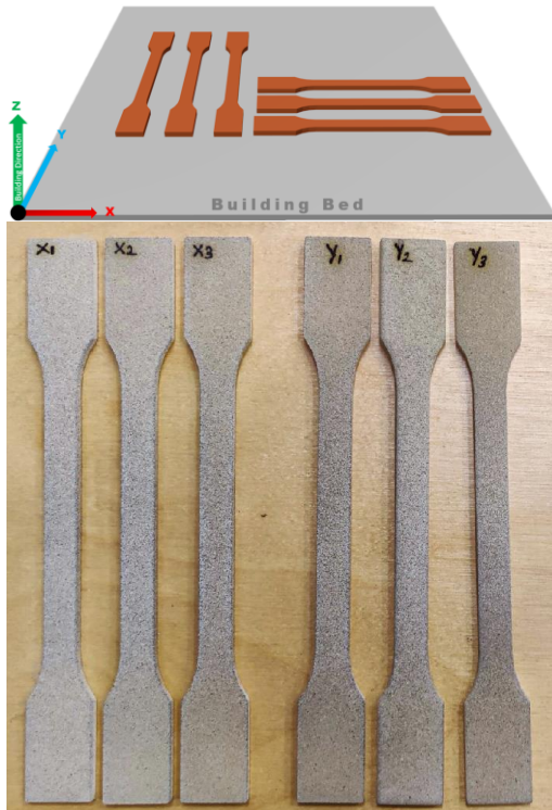
Fig. 4. Layout view on building table and specimens
