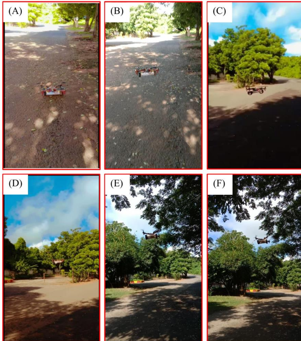
Fig. 10. Snapshots of aerial motion control-based experimental results of a combined vehicle (UAV + UGV), (UAV, unmanned aerial vehicle; UGV, unmanned ground vehicle)
