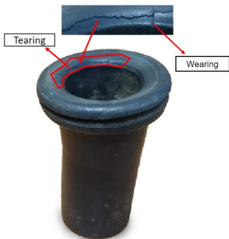
Fig. 1. Damaged textile machine yarns pass analyzed
