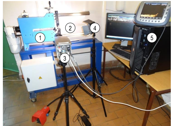
Fig. 7. Experimental test stand: 1 – shear slitting machine, 2 – sheet, 3 – i-SPEED TR camera, 4 – light source and 5 – PC
