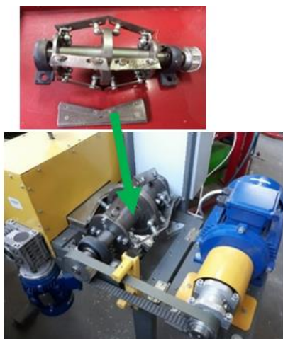
Fig. 10. Mounted design of the cutting drum of the conical type in the chaff cutter
