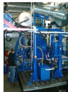
Fig. 7. Test engine for calibration of calculation model
