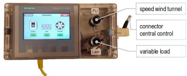
Fig. 6. Remote control of wind tunnel and central control unit
