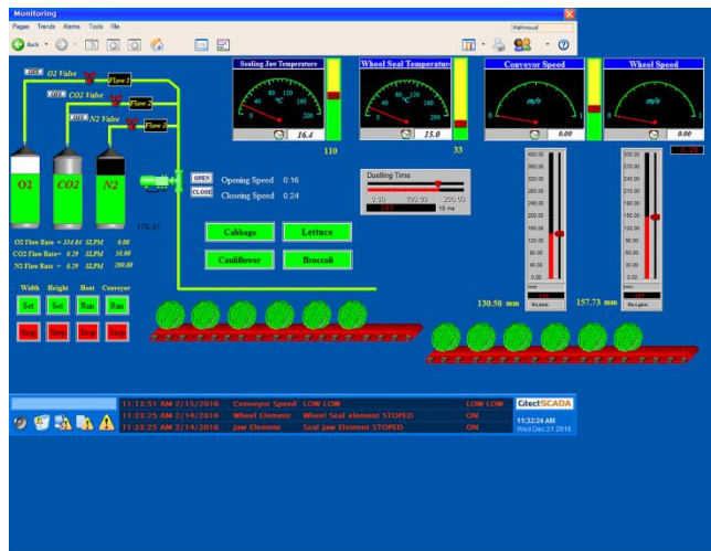
Fig. 7. The graphic page designed for the HFFS system. HFFS, horizontal form-fill-seal
