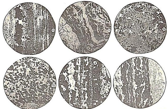
Fig. 2. Formations of magnetite (black) with other minerals (enlarged 40 times): (a) interspersed structure of magnetite grains; (b) replacement of magnetite with quartz; (c) relics of quartz and iron mica in the magnetite layer; (d) folded jaspilite; (e) development of cummingtonite in the ore layer; (f) replacement of magnetite with aegirine
