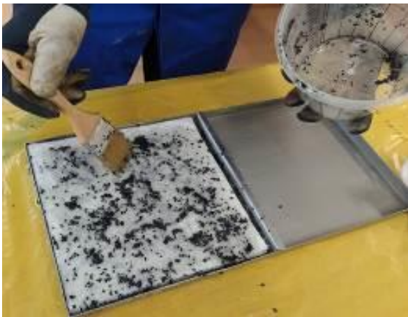
Fig. 6. Manufacture of materials by hand lamination
