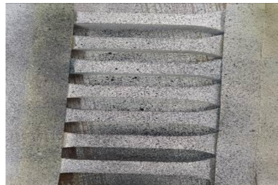
Fig. 8. Samples prepared for measurements using the ARAMIS SRX system
