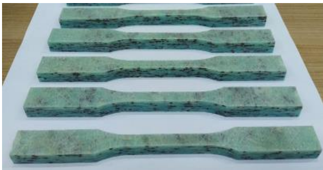
Fig. 7. Test samples cut by water cutting
