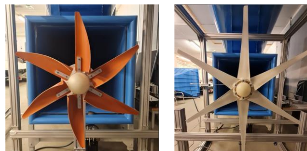
Fig. 4. Horizontal rotors: drag-type rotor (left) and lift-type rotor (right)
