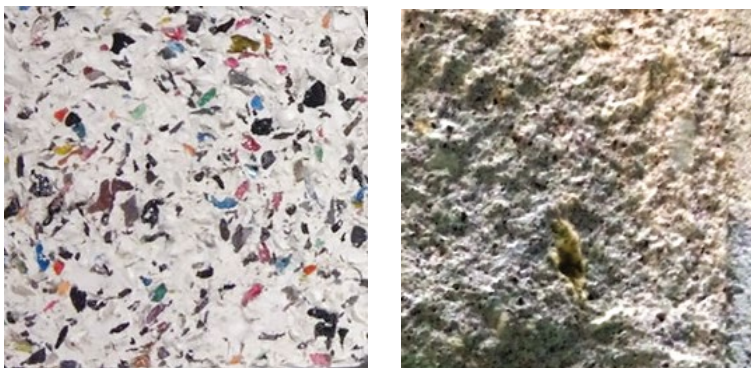
FIG. 5.2. Left: Plasterboard with plastic cable waste additives. Right: Cement mortar with mineral wool waste (Source: photos by A. Vidales Barriguete, 2020)
