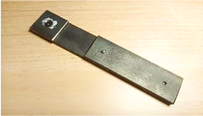
FIG. 2. S235 steel plates about dimensions 100x30x4 fastened by blind rivet Al-A2 4 × 12
