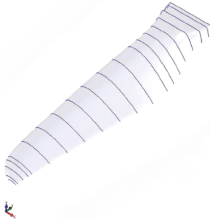
FIG. 6. View of the upper surface stretched on previously generated 3D curves [10]
