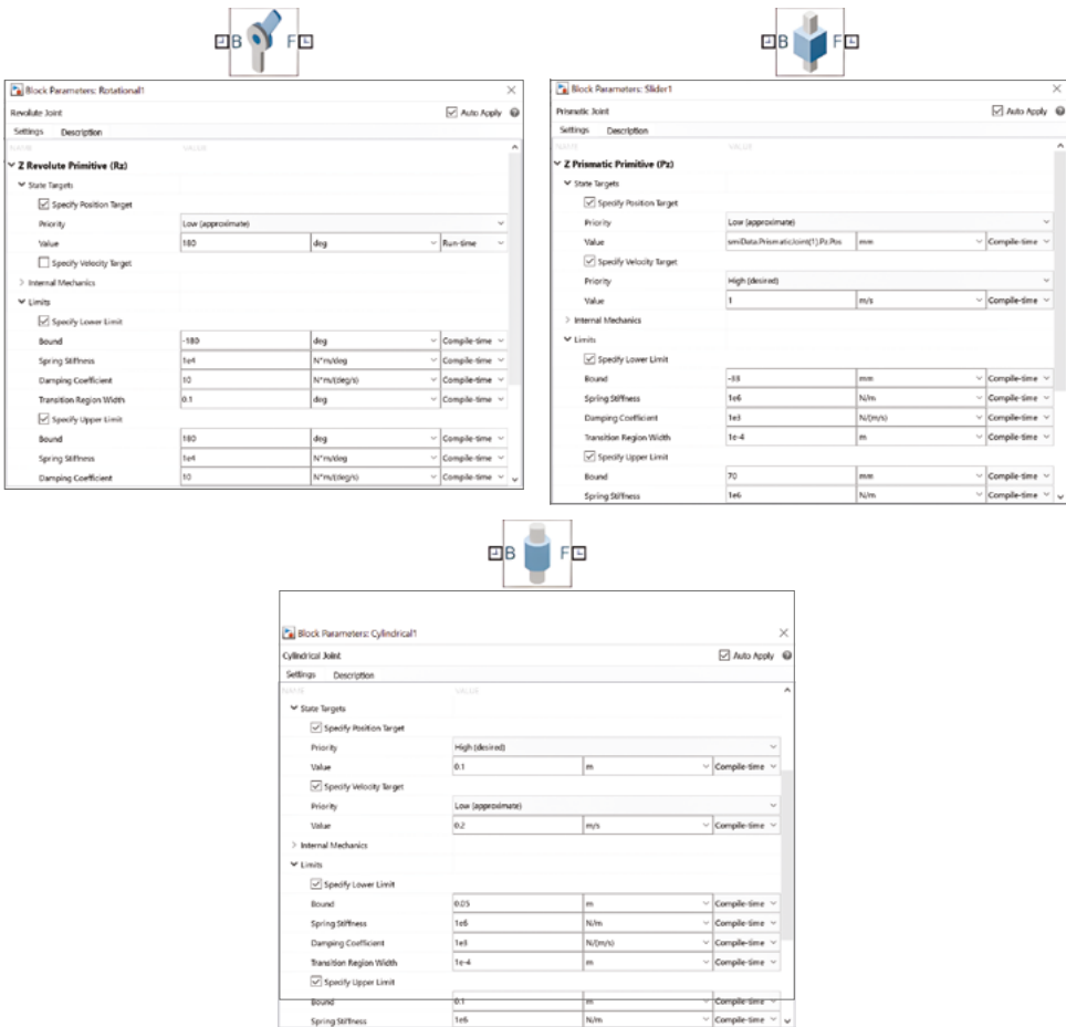
FIG. 7. Description of connection block models and their properties in the MATLAB Simulink
