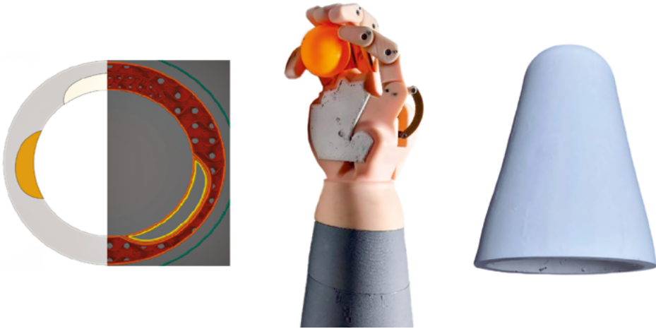
FIG. 3. Transition from a CAD model with parametric elements to a slicer with added settings for the density of individual objects, along with examples of application in hand bioprosthetics and prosthetic socket
