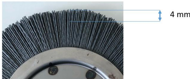
Fig. 6. Place of measurement of bristle thickness after the test
