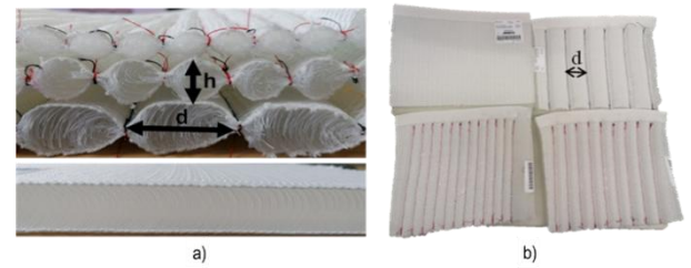
Fig. 2 Spacer fabric variations for experimental testing: (a) cross view, (b) top view; h cushion height, d seam distance
