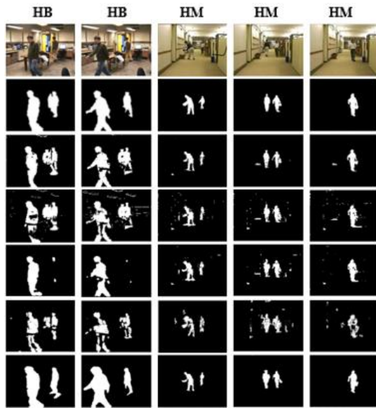
Fig. 7. Comparative analysis of our approach with state-of-the-art methods by exploiting specific videos such as “HumanBody1-HB” and “HallAndMonitor-HM” from the SBI2015 dataset. The left-to-right layout shows results for: original, ground truth, DeepBS [27], SC_SOBS [25], SuBSENSE [24], GMM_Zivk [26], as well as our method. The results for NThr=4 are displayed in this figure
